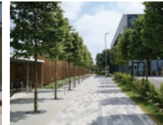
BLOCK PAVING DESIGN INTEGRATING SOFT LANDSCAPING TO DEFINE AND PRIORITISE PED/CYCLE ROUTES
